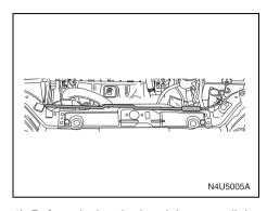
4) Before closing the hood, be sure all the filler caps are on properly. Then lift the hood to relieve pressure on the hood prop. Remove the hood prop from the slot in the hood and return the prop to its retainer. Lower the hood 12 in (30 cm) above the vehicle and release it to latch fully. Check to make sure the hood is closed and repeat the process if necessary.
